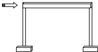
For this simple portal frame (RC or Steel), set-up the foundation system (under investigation), portal frame, simple loading frame + device (not shown), way to measure the horizontal deflection of the frame. Just by recording the horizontal push (by jacks) and measuring the displacement, we can plot the load-deflection curve.
